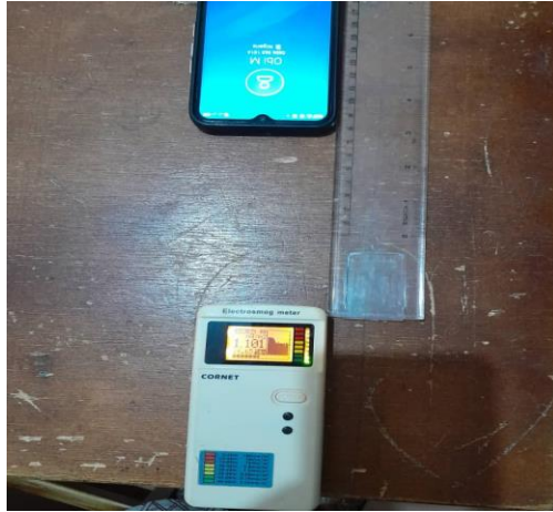
Figure 1. Power density measurement set-up.
